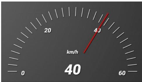
Speed: Shows velocity based on the GPS antenna data. As many other gauges, can be metric or imperial and colors, angles and sizes can be customized.
