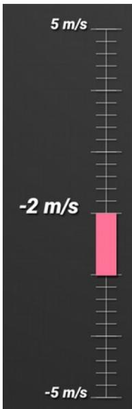
Vertical Speed: Shows the vertical speed of the path, or rate of ascent.
