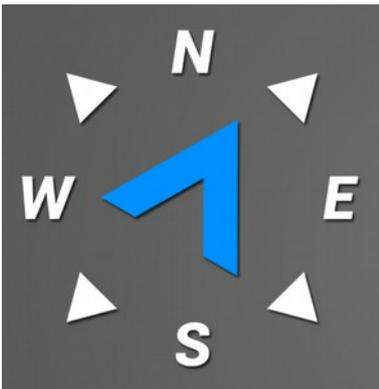
Course Direction: Points at the cardinal direction the device is moving to, not necessarily the direction it is looking at.
